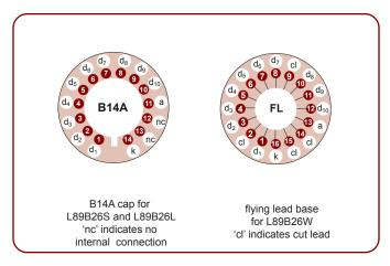
A range of B14A sockets is available to suit the B14A cap of the L89B26S and L89B26L. The socket range includes versions with or without a mounting flange, and with contacts for mounting directly onto printed circuit boards.
